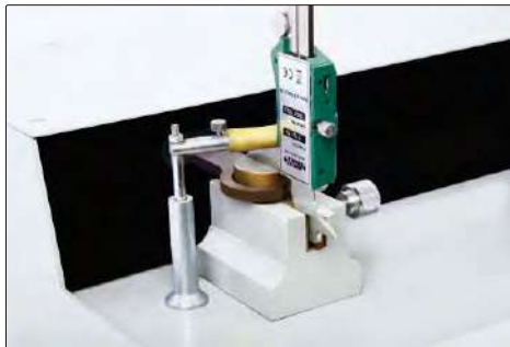
lapping measuring surfaces of caliper lower jaws
