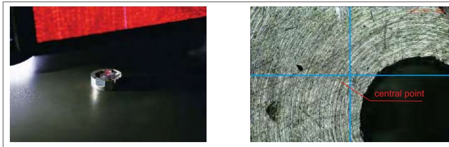
laser indicator locates the central point
