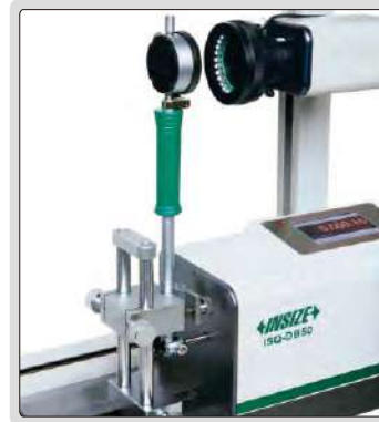
check bore gages
