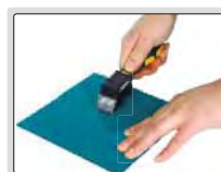
step 1: make grid cutting on surface
