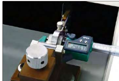
lapping measuring surfaces of outside micrometer
